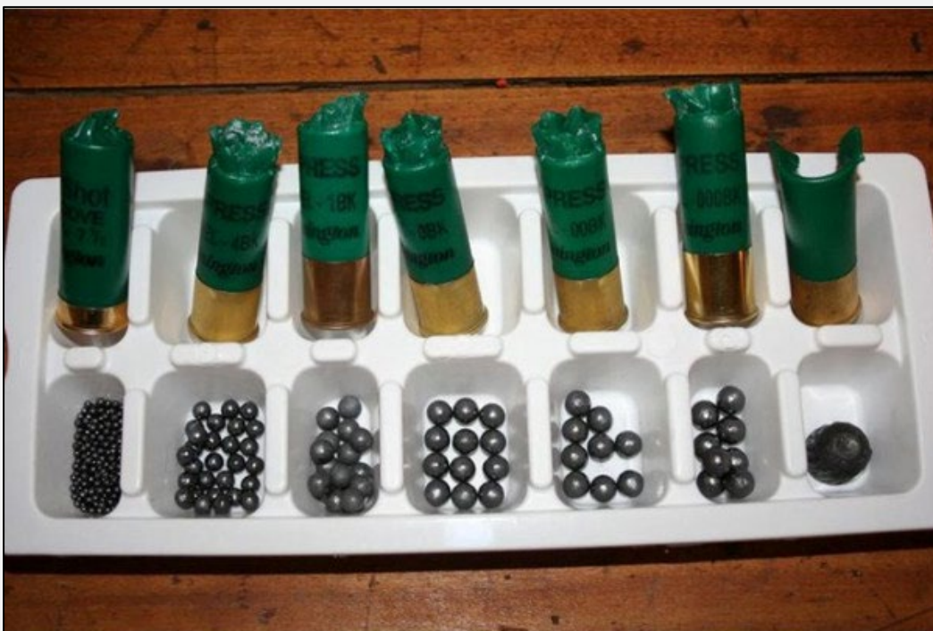
▲ 12 gauge shotgun cartridges with variety of metal projectiles
