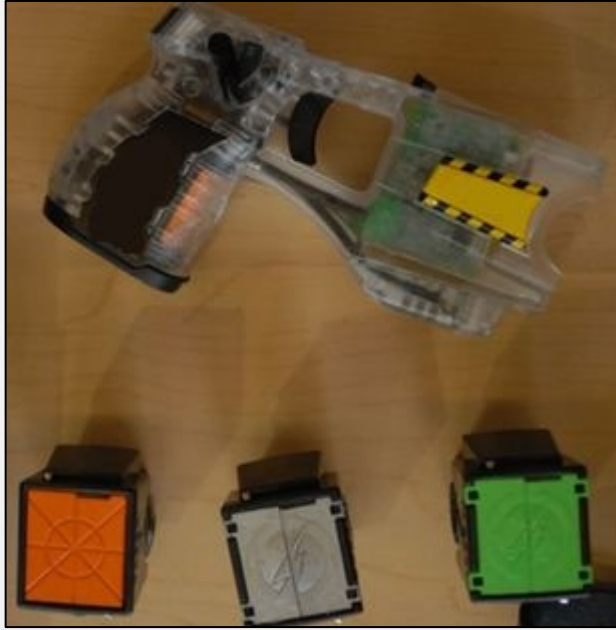
▲ Projectile stun gun with cartridges of different ranges
