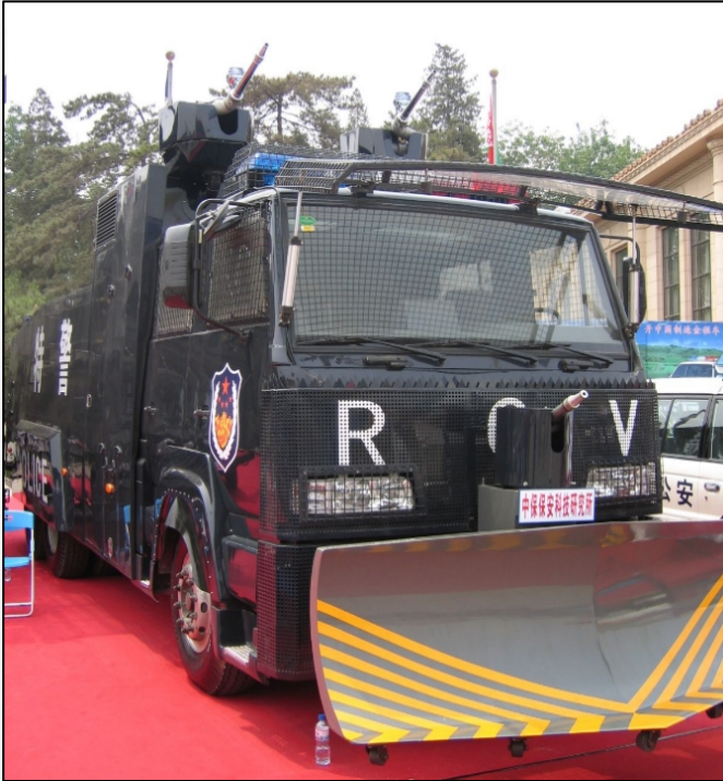
◀ Water cannon mounted on large crowd control vehicle
