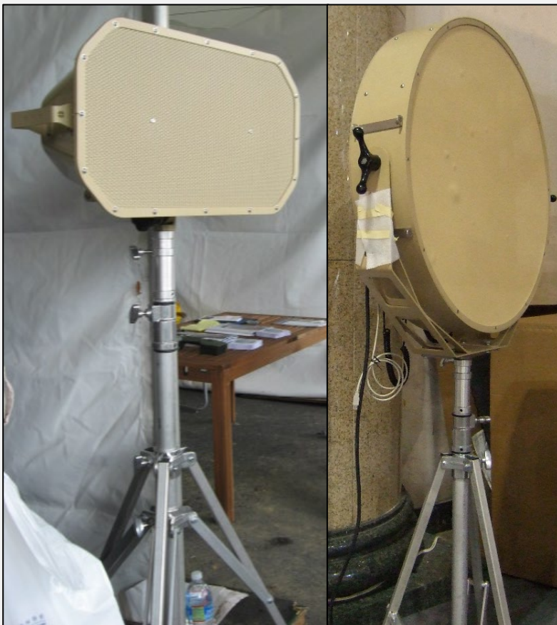
◀ Free-standing acoustic hailing device
