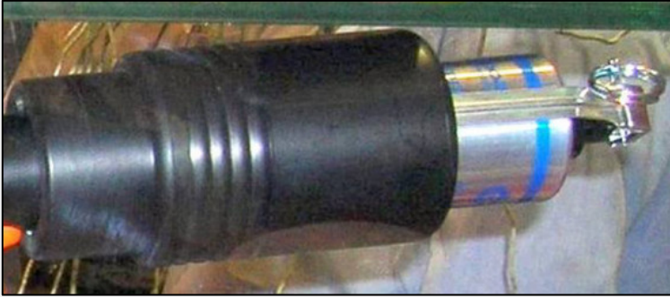
▲ Launching cup with 38mm grenade
