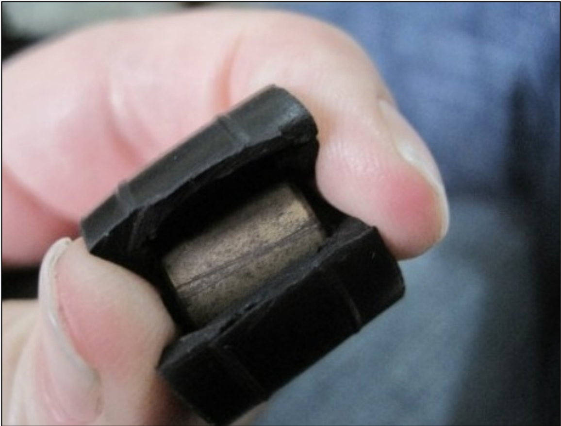
▲ Rubber coated metal bullet showing metal core
